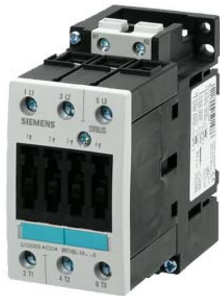
CONTACTOR, AC-3 22 KW/400 V, AC 48V 50/60HZ, 3-POLE, SIZE S2, SCREW CONNECTION MOUNTING POSITION VERTICAL
