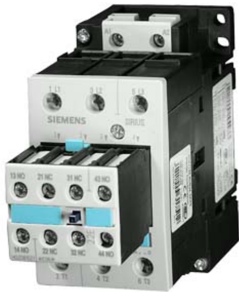
CONTACTOR, AC-3 22 KW/400 V, AC 230V 50/60HZ 2 NO + 2 NC 3-POLE, SIZE S2, SCREW CONNECTION
