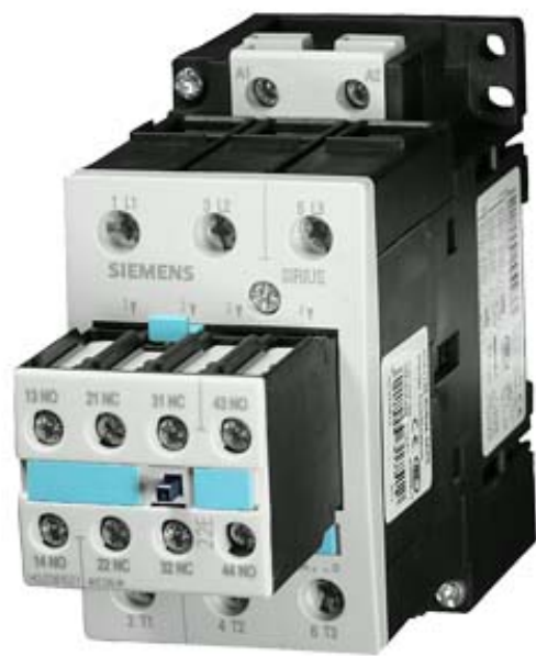
CONTACTOR, AC-3 22 KW/400 V, AC 220V 50/60HZ 2 NO + 2 NC 3-POLE, SIZE S2, SCREW CONNECTION
