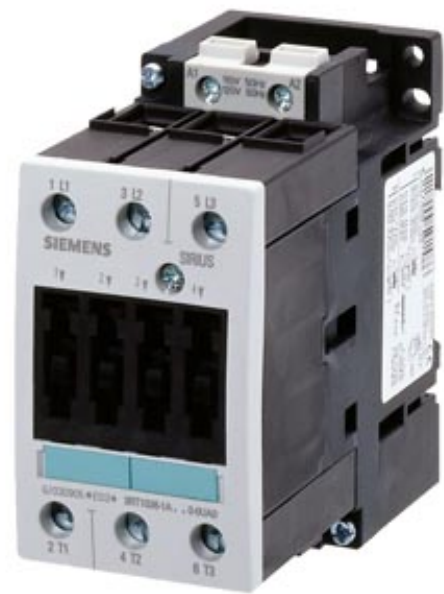
CONTACTOR, AC-3 22 KW/400 V, AC 230 V, 50 HZ, 3-POLE, SIZE S2, SCREW CONNECTION MOUNTING POSITION VERTICAL
