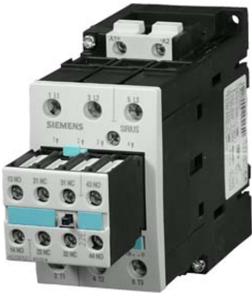
CONTACTOR, AC-3 22 KW/400 V, DC 125 V, 3-POLE, 2 NO + 2 NC, SIZE S2, SCREW CONNECTION
