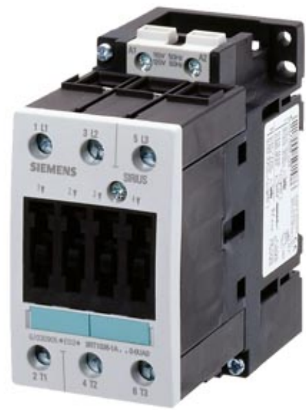
CONTACTOR, AC-3 22 KW/400 V, DC 230 V, 3-POLE, SIZE S2, SCREW CONNECTION
