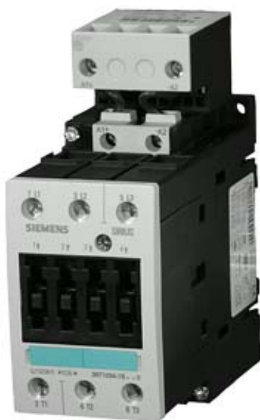
CONTACTOR, AC-3 22 KW/400 V, AC110V 50/60HZ 3-POLE, SIZE S2, SCREW CONNECTION
