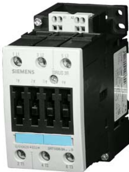
CONTACTOR, AC-3 22 KW/400 V, AC 100 V, 50 HZ/100...110V,60HZ 3 POLE, MOD. S2, CAGE CLAMP
