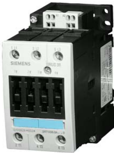
CONTACTOR, AC-3 22 KW/400 V, AC 48 V, 50 HZ, 3-POLE, SIZE S2, CAGE CLAMP
