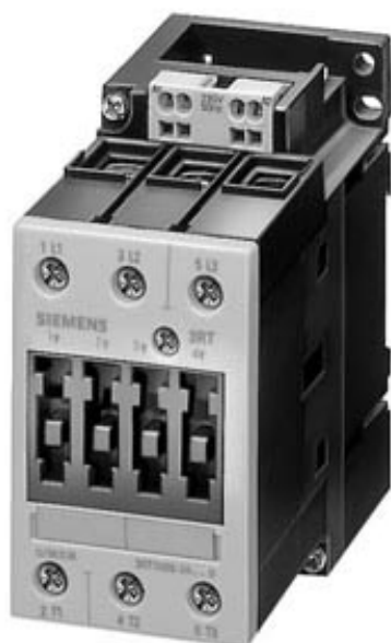
CONTACTOR, AC-3 22 KW/400 V, AC 220 50/60 HZ, 3-POLE, SIZE S2, CAGE CLAMP
