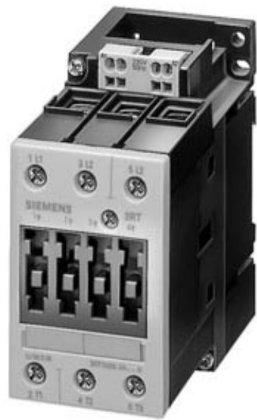
CONTACTOR, AC-3 22 KW/400 V, AC 230 V, 50 HZ, 3-POLE, SIZE S2, CAGE CLAMP
