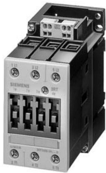
CONTACTOR, AC-3 22 KW/400 V, DC 24 V, 3-POLE, SIZE S2, CAGE CLAMP
