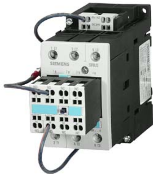
CONTACTOR, AC-3, 22KW/400V, DC 72V, 0.7...1.25*US, 3-POLE, SZ. S2, CAGE CLAMP CONNECTION
