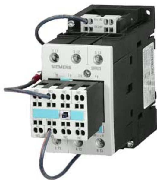
CONTACTOR, AC-3, 22KW/400V, DC 52V, 0.7...1.25*US, 3-POLE, SIZE S2, CAGE-CLAMP CONNECTION
