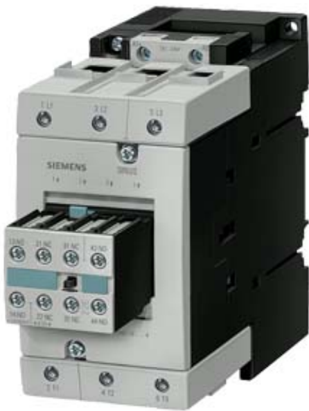
CONTACTOR, AC-3 30 KW/400 V, AC 24 V, 50 HZ, 2 NO + 2 NC 3-POLE, SIZE S3, SCREW CONNECTION
