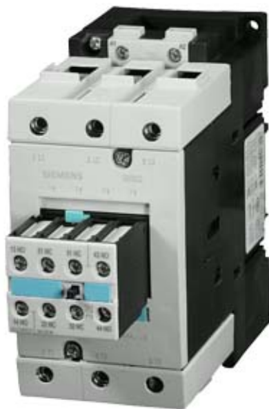
CONTACTOR, AC-3 30 KW/400 V, AC 42V 50/60HZ, 2 NO + 2 NC, 3-POLE, SIZE S3, SCREW CONNECTION
