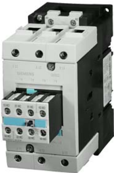
CONTACTOR, AC-3 30 KW/400 V, AC 110V 50HZ/120V 60HZ 2 NO + 2 NC 3-POLE, SIZE S3 SCREW CONNECTION
