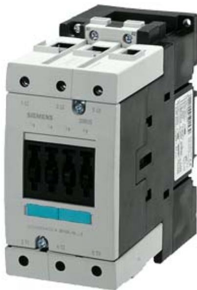
AC-3 CONTACTOR, 30 KW/400 V, 220 V 60 HZ AC, 3-POLE, SIZE S3, SCREW TERMINAL
