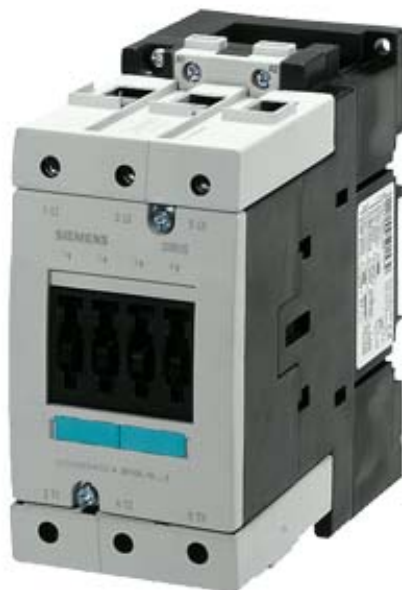
CONTACTOR, AC-3 30 KW/400 V, AC 400 V, 50 HZ, 3-POLE, SIZE S3, SCREW CONNECTION
