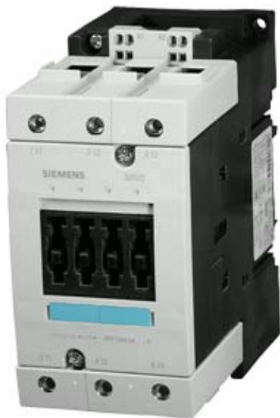
CONTACTOR, AC-3 30 KW/400 V, AC 220 V 50/60 HZ, 3-POLE, SIZE S3, CAGE CLAMP
