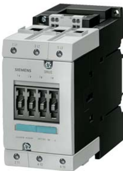
CONTACTOR, AC-3 30 KW/400 V, DC 60 V, 3-POLE, SIZE S3, CAGE CLAMP
