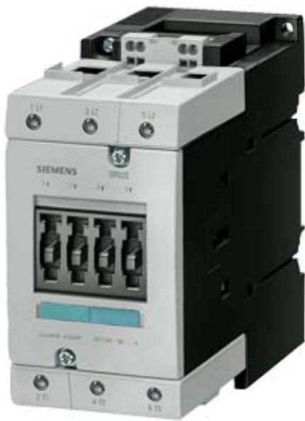
CONTACTOR, AC-3 30 KW/400 V, DC 48 V, 3-POLE, SIZE S3, CAGE CLAMP
