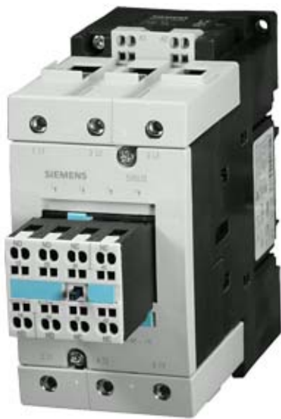
CONTACTOR, AC-3 30 KW/400 V, AC 230 V 50/60 HZ, 3-POLE, SIZE S3, 2NO/2NC CAGE CLAMP, WITH BUILT-IN RC ELEMENT
