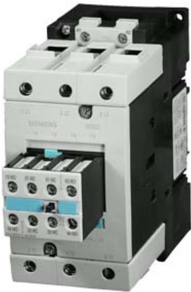
CONTACTOR, AC-3 37 KW/400 V, AC 48 V, 50/60 HZ, 2 NO + 2 NC 3-POLE, SIZE S3, SCREW CONNECTION
