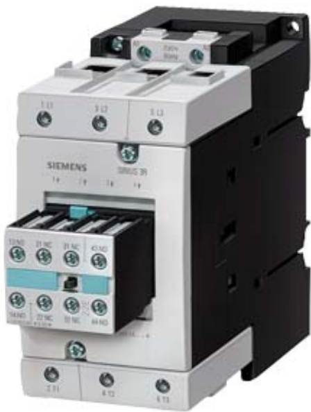
CONTACTOR, AC-3 37 KW/400 V, AC 230 V, 50 HZ, 2 NO + 2 NC 3-POLE, SIZE S3, SCREW CONNECTION
