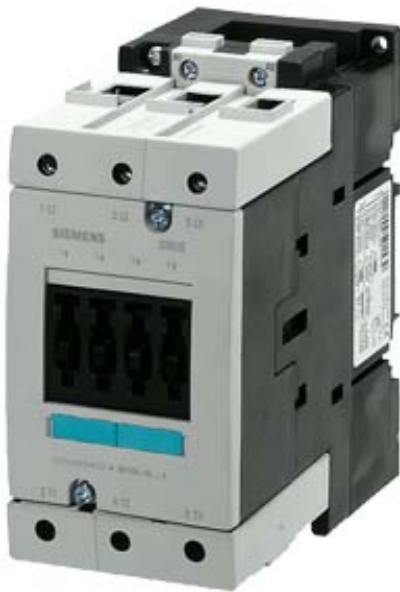
CONTACTOR, AC-3 37 KW/400 V, AC 400 V, 50 HZ, 3-POLE, SIZE S3, SCREW CONNECTION
