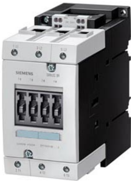
CONTACTOR, AC-3 37 KW/400 V, AC 42V, 50/60HZ, 3-POLE, SIZE S3, CAGE CLAMP
