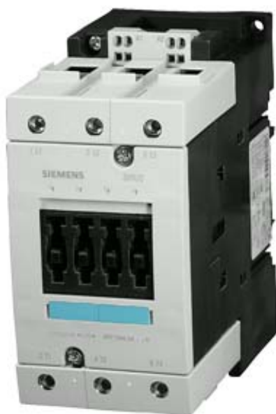
CONTACTOR, AC-3 37 KW/400 V, AC 110 V 50/60 HZ, 3-POLE, SIZE S3, CAGE CLAMP
