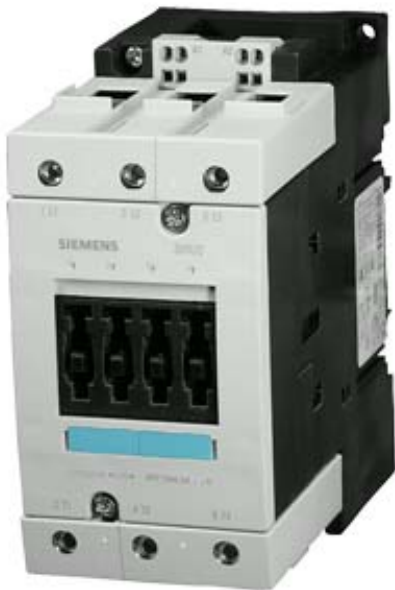
CONTACTOR, AC-3 37 KW/400 V, AC 230 V 50/60 HZ, 3-POLE, SIZE S3, CAGE CLAMP
