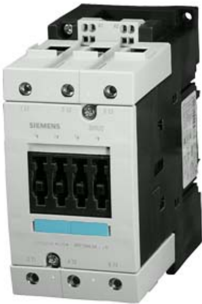
CONTACTOR, AC-3 37 KW/400 V, AC 400 V, 50 HZ, 3-POLE, SIZE S3, CAGE CLAMP
