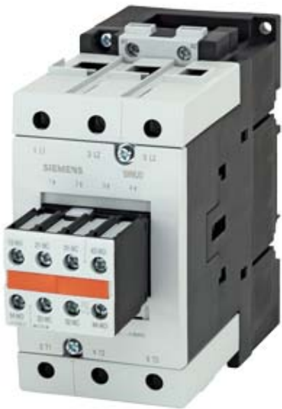
CONTACTOR, AC-3, 45KW/400V, AC 120V, 60HZ, 2NO+2NC, JOINTED 3-POLE, SIZE S2. SCREW TERMINAL
