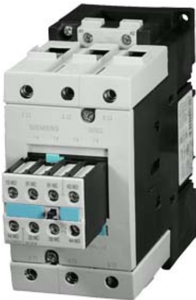
CONTACTOR, AC-3 45 KW/400 V, AC 110V 50HZ/120V 60HZ 2 NO + 2 NC , 3-POLE, SIZE S3, SCREW CONNECTION
