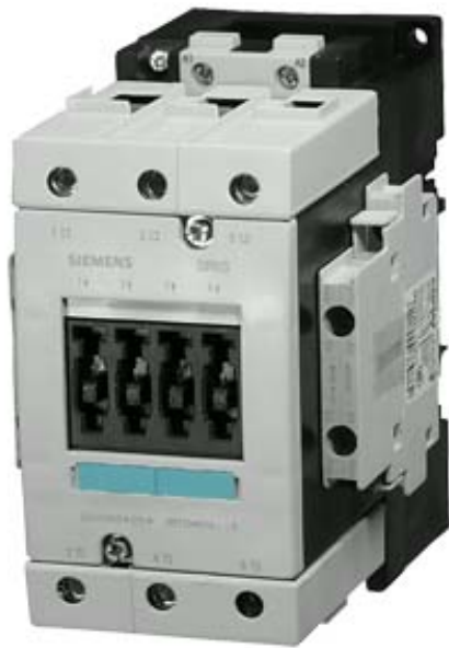
CONTACTOR, 3PH, 45KW/400V, 230V AC 50/60HZ, 2NO+2NC, 2NO + 2NC, LATERAL, 3-POLE, SIZE S3, SCREW TERMINAL
