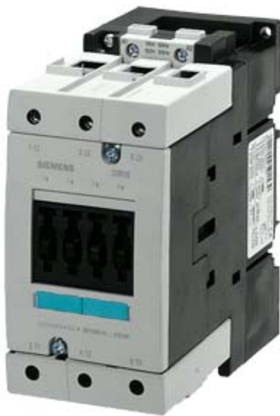
CONTACTOR, AC-3 45 KW/400 V, AC 220V 50HZ/240V 60HZ 3-POLE, SIZE S3, SCREW CONNECTION
