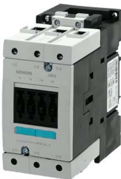
CONTACTOR 3-PH 45 KW/400 V, 500 V AC 50/60 HZ 3-POLE, SIZE S3, SCREW CONNECTION
