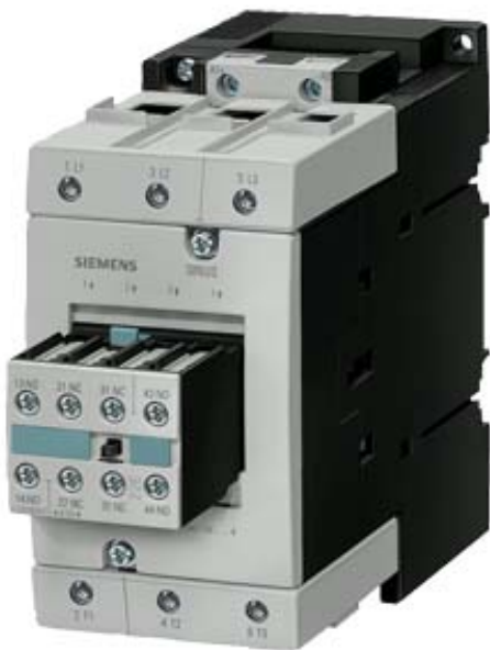
CONTACTOR, AC-3 45 KW/400 V, DC 220 V, 2 NO + 2 NC, 3-POLE, SIZE S3, SCREW CONNECTION
