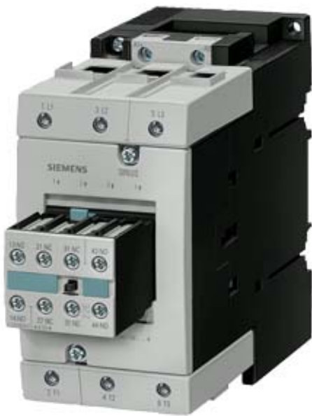
CONTACTOR, AC-3 45 KW/400 V, DC 48 V, 2 NO + 2 NC, 3-POLE, SIZE S3, SCREW CONNECTION
