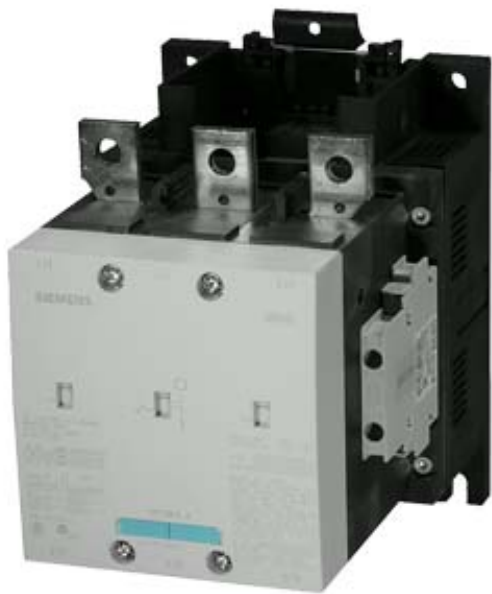
VAC. CONTACTOR, 132KW/400V/AC-3 WITHOUT COIL AUXILIARY CONTACTS 2NO+2NC 3-POLE, SIZE S10 RAIL CONNECTIONS
