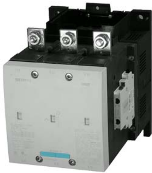
VAC. CONTACTOR, 250KW/400V/AC-3 WITHOUT COIL AUXILIARY CONTACTS 2NO+2NC 3-POLE, SIZE S12 RAIL CONNECTIONS
