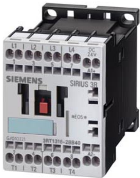
CONTACTOR, AC-3 4 KW/400 V, AC-1 18 A, DC 220 V, 4-POLE, 4 NO, SIZE S00, CAGE CLAMP CONNECTION
