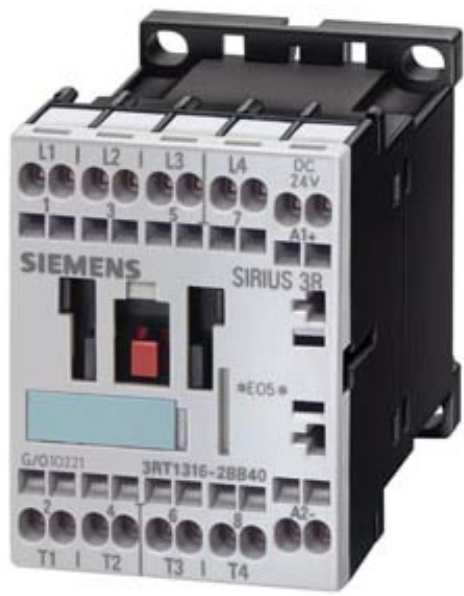
CONTACTOR, AC-3 4 KW/400 V, AC-1 18 A, DC 230 V, 4-POLE, 4 NO, SIZE S00, CAGE-CLAMP CONNECTION
