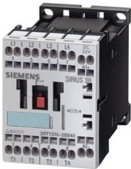
CONTACTOR, AC-3 4 KW/400 V, AC-1 18 A, DC 48 V, 4-POLE, 4 NO, SIZE S00, CAGE-CLAMP CONNECTION
