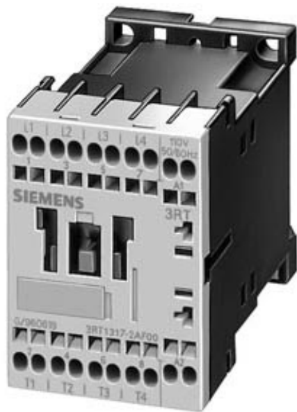
CONTACTOR, AC-3 5.5KW/400 V, AC-1 22 A, AC 24 V, 50 HZ, 4-POLE, 4 NO, SIZE S00, CAGE CLAMP CONNECTION
