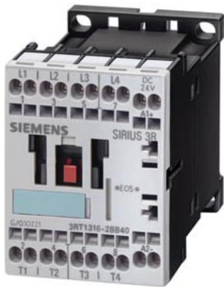
CONTACTOR, AC-3 5.5KW/400 V, AC-1 22 A, DC 42 V, 4-POLE, 4 NO, SIZE S00, CAGE-CLAMP CONNECTION
