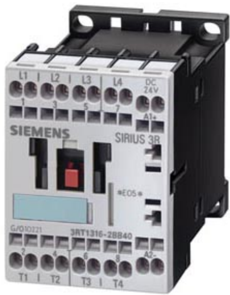
CONTACTOR, AC-3 5.5KW/400 V, AC-1 22 A, DC 110 V, 4-POLE, 4 NO, SIZE S00, CAGE-CLAMP CONNECTION
