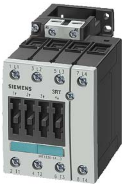
CONTACTOR, AC-1 60 A, AC 48 V 50/60 HZ 4-POLE, SIZE S2, SCREW CONNECTION AVAILABLE MARCH '98
