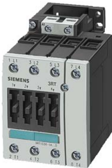
CONTACTOR, AC-1 60 A, AC 208 V 60 HZ 4-POLE, SIZE S2, SCREW CONNECTION
