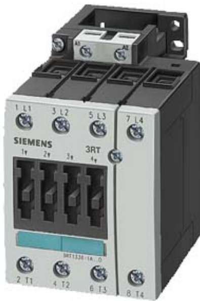
CONTACTOR, AC-1, 55 A, 220 V AC, 50/60 HZ, 4-POLE, 4 NO, SIZE S2 SCREW CONNECTION
