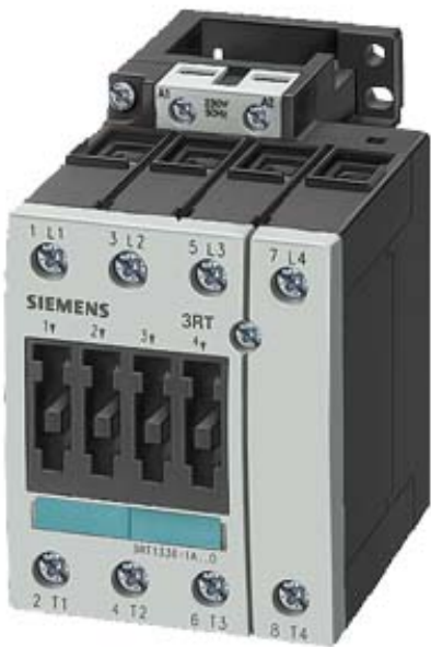
CONTACTOR, AC-1 60 A, DC 42 V, 4-POLE, SIZE S2, SCREW CONNECTION AVAILABLE MARCH '98
