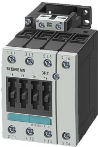
CONTACTOR, AC-1 60 A, DC 110 V, 4-POLE, SIZE S2, SCREW CONNECTION
